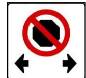
No stopping on either side of the sign.
